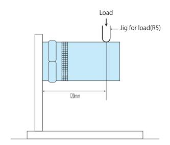
Determine the shape of the hinge starts to change under load as adove.
